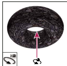
The 3D Orbit tool orbits the camera in the x or y direction (moves the camera, not the object).
