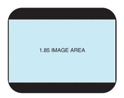
One option is called letterboxing. The top and bottom of the 1.33 television screen are not used, allowing the film's proper aspect ratio to appear in the middle of the TV screen. The narrow black bands on the top and bottom of the 1.33 television screen alter the screen's aspect ratio to 1.85:1. Many television viewers find letterboxing unacceptable because parts of the screen are blank.
