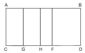
This divides the frame into four unequal parts. The proportional relation of CF to FD is called the golden section. CG is the same ratio to CF as FD is to CF. HF has the same ratio to GH as CG is to GF.
