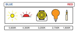
The Kelvin scale helps us describe and compare the color of light emitted from various sources. The lower the Kelvin number the redder the light, and the higher the Kelvin number the bluer the light. The scale is calibrated in degrees although these degree numbers as we use them in lighting have nothing to do with thermal heat. A 5,600 K light is not necessarily hotter than a 2,700 K light.
