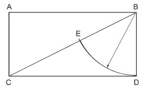
First, divide the frame in half with a diagonal line CB. Then transfer the length of the frame's side BD onto the diagonal line creating EB.
