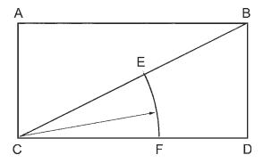
Now, transfer the length of CE down to the bottom of the frame creating point F.
