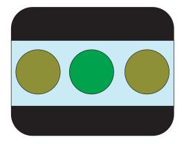
The first solution is letterboxing. A 2.40:1 aspect ratio cannot fit onto a 1.33:1 screen unless large horizontal bands at the top and bottom of the screen remain unused. General audiences won't accept letterboxing because so much of the 1.33 television screen remains blank.
