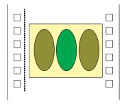
This is the same shot as it will appear on the 35 mm film. The image has been squeezed by the camera's anamorphic lens to fit onto the standard 1.33:1 35 mm film frame.
