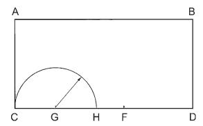
Transfer the length of CG across the bottom of the frame creating point H. Draw vertical lines from points G, H and F.
