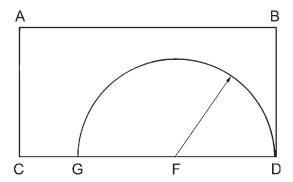
Transfer the length of FD across the bottom of the frame creating point G.
