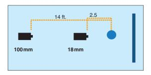
This is an overhead view or ground plan of a wall, an actor (indicated by the dot) and a camera. The camera, with a 100 mm telephoto lens, is set up 14 feet from an actor in front of a wall, but the wall is out of focus and we want both the actor and the wall to be in focus. Without moving the camera we switch to an 18 mm wide angle lens that we think "has a much greater depth of field."
